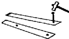
9. With a small nail, hammer a hole in each piece near one end. Hammer one more hole in one piece about 2.5-cm. from the other end.
