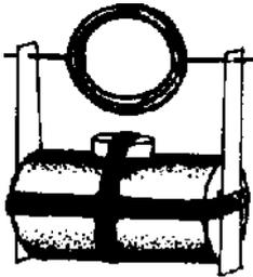
13. Now pull the metal strips a little apart and slip the motor coil in their holes.
