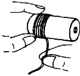
2. Take 1-metre of Copper wire (20 gauge). Straighten it by running it through a piece of cloth. Wind it tightly on a torch battery. The loops of the wire should be adjacent to one another. They should not overlap. The coil should have about 10 turns.
