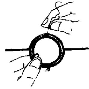
4. Tie the coil at several places with little bits of string. The string will keep the loops of the coil in place.
