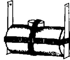
12. The metal strips serve three purposes. They act as power leads, supplying current to the coil. They are also bearing supports for the coil. Finally, they also make a stand for the motor.
