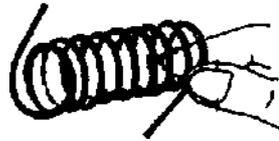
3. When the coil is removed from the battery it opens up like a spring.
