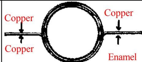
7. The copper / enamel sequence leads to make / break of the circuit. This **BRUSH** or **COMMUTATOR** is the heart of this simple motor. If all the enamel is removed from the end leads then the motor will not work. The coil is now ready.
