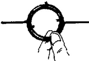
5. The two ends of the coil should jut diametrically outwards. The coil will rotate on these two ends. So, ensure symmetry and even distribution of the coil's weight.
