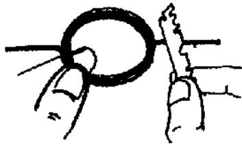
6. Now, scrape the enamel from three sides of the end leads using a blade. The enamel will remain only on the bottom of the end leads.
